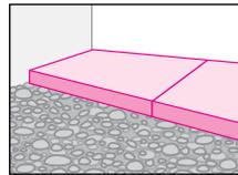
**1. LAYING GRAVEL.** Lay at least 4" (102mm) of coarse, clean gravel on the top of the undisturbed soil and ensure that it is level.
