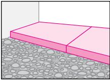
**1. INSTALLING C-300.** Install C-300 over appropriate substrate. Ensure panels are butted together as tight as possible. It's suggested that all joints are taped with approved Owens Corning® JointSealR® tape.
