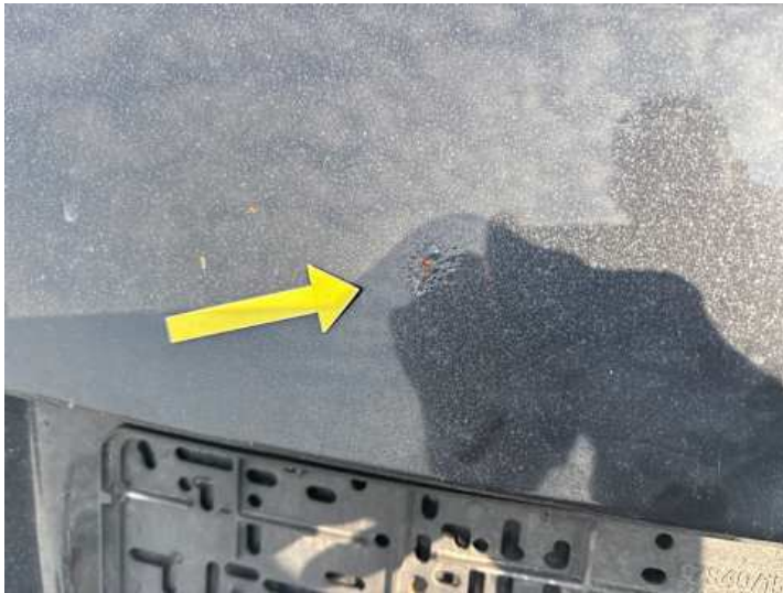
Heckklappe (Lackschaden, Rost)
