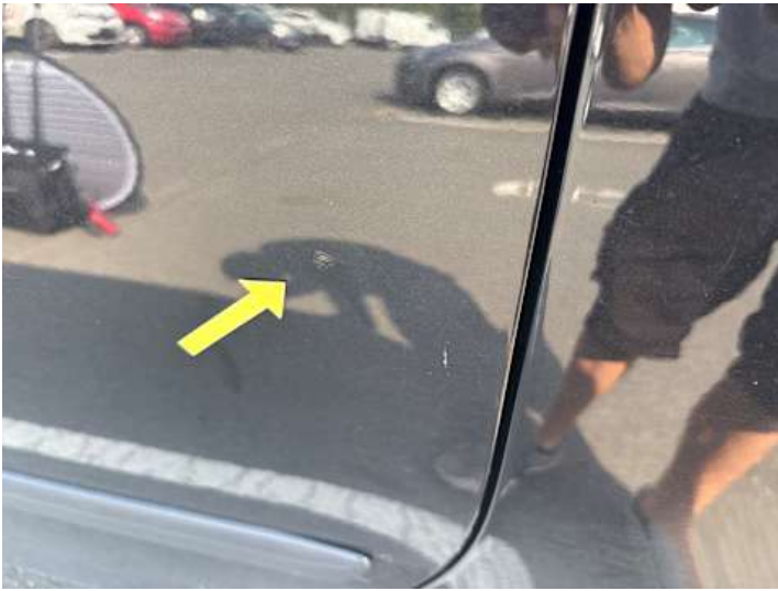
Türe hinten links (Lackschaden, Rost)
