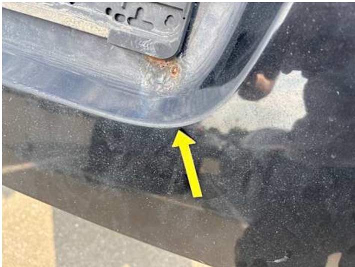
Heckklappe (Lackschaden, Rost)
