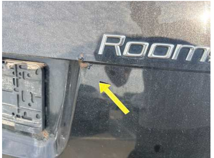
Heckklappe (Lackschaden, Rost)
