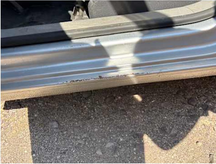
Schweller links (Lackschaden, Rost)
