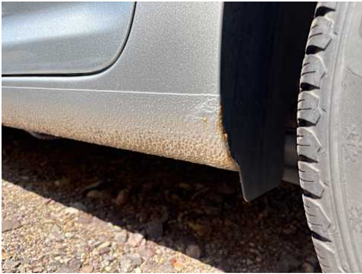
Schweller links (Lackschaden, Rost)
