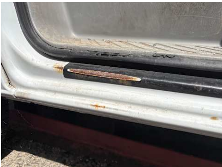
Schweller links (Lackschaden, Rost)
