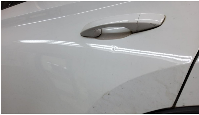
Tür hinten links - SmartRepair
