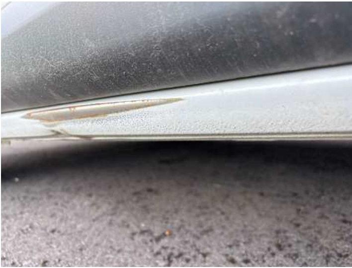
Schweller links (Lackschaden, Rost)
