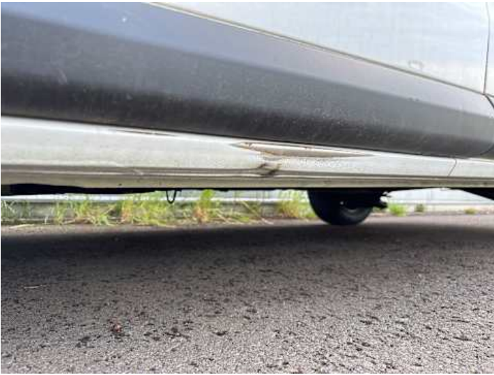
Schweller links (Lackschaden, Rost)
