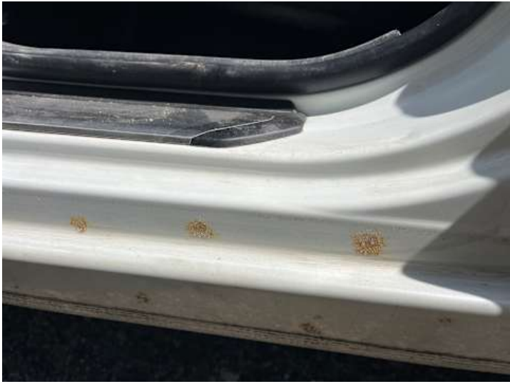
Schweller links (Lackschaden, Rost)
