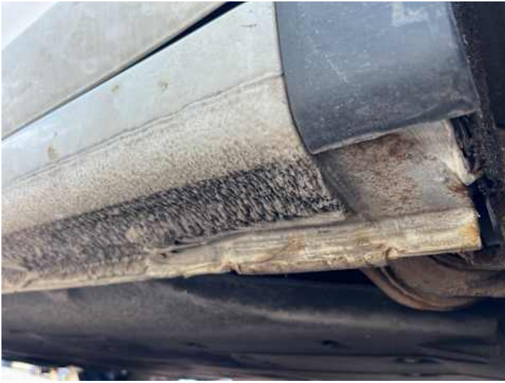
Schweller links (Lackschaden, Rost)
