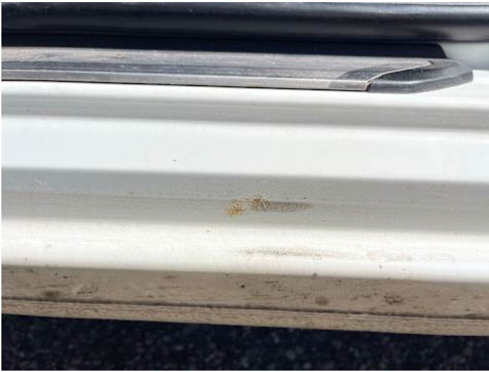
Schweller links (Lackschaden, Rost)
