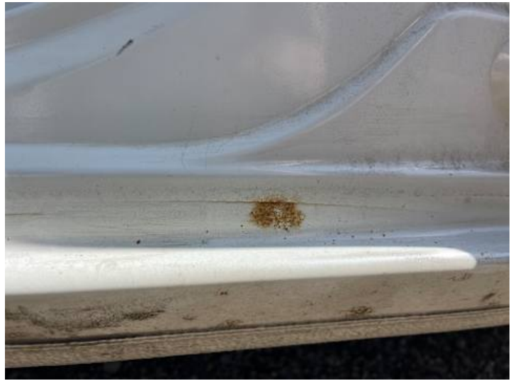
Schweller links (Lackschaden, Rost)
