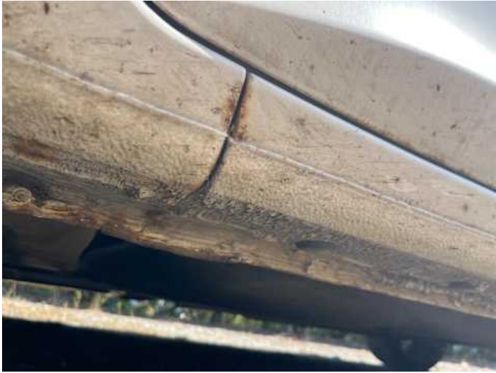
Schweller links (Lackschaden, Rost)
