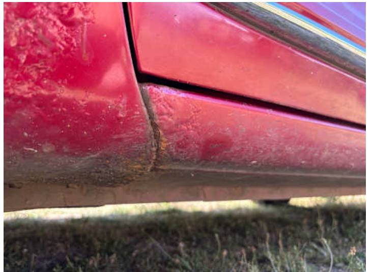
Schweller links (Lackschaden, Rost)
