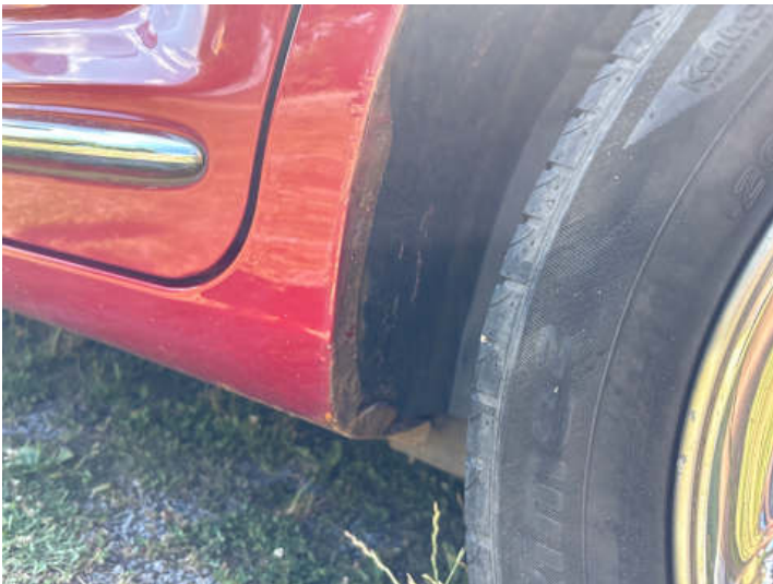
Schweller links (Lackschaden, Rost)
