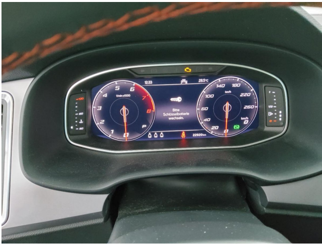
Schlüsselbatterie defekt (DEKRA)
