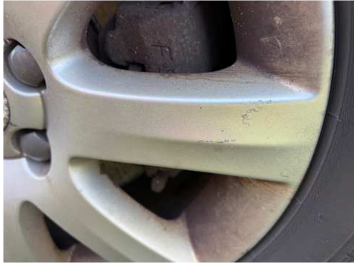
Rad (vehicle.damage-label.porous, Rost)
