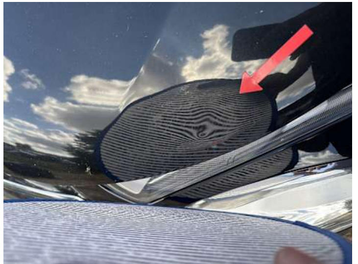
Motorhaube (Delle, Rost)
