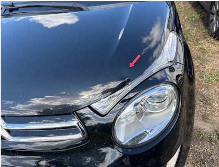
Motorhaube (Delle, Rost)
