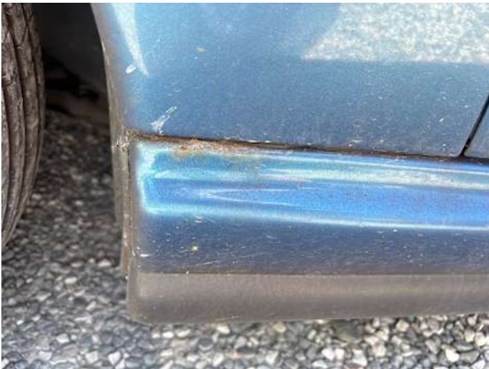
Schweller links (Lackschaden, Rost)
