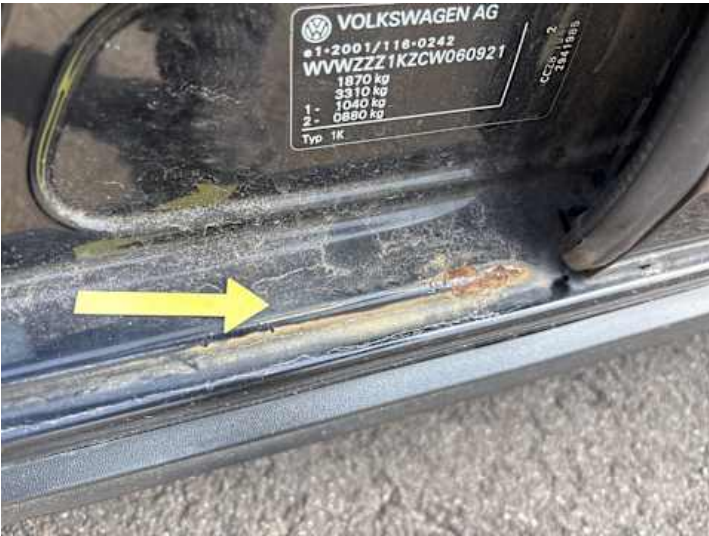
Schweller links (Lackschaden, Rost)
