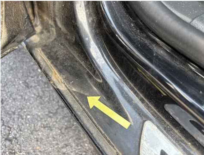
Schweller links (Lackschaden, Rost)
