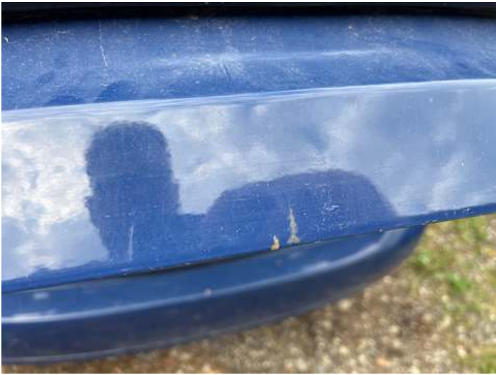
Heckklappe (Lackschaden, Rost)
