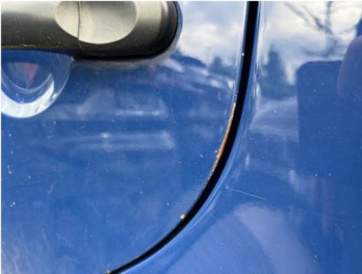
Türe hinten links (Lackschaden, Rost)
