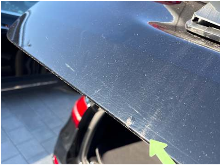
Heckklappe (Lackschaden, Rost)
