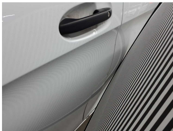
Beschädigung #6: Tür vorn links: Tür - Delle(n) - Smart Repair
