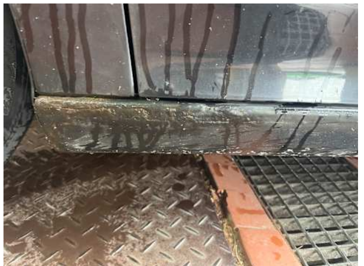
Schweller links (Lackschaden, Rost)
