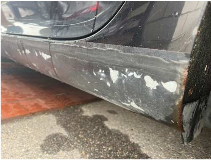
Schweller links (Lackschaden, Rost)
