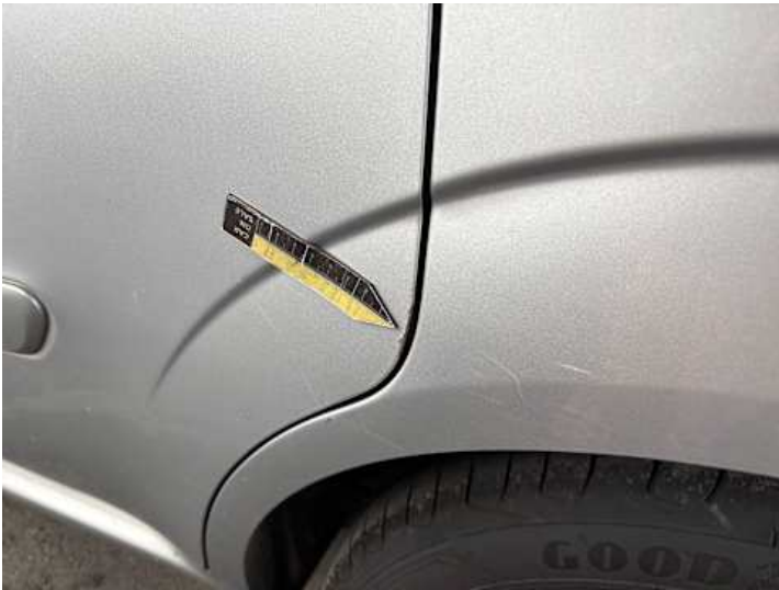
Türe hinten links (Lackschaden, Rost)
