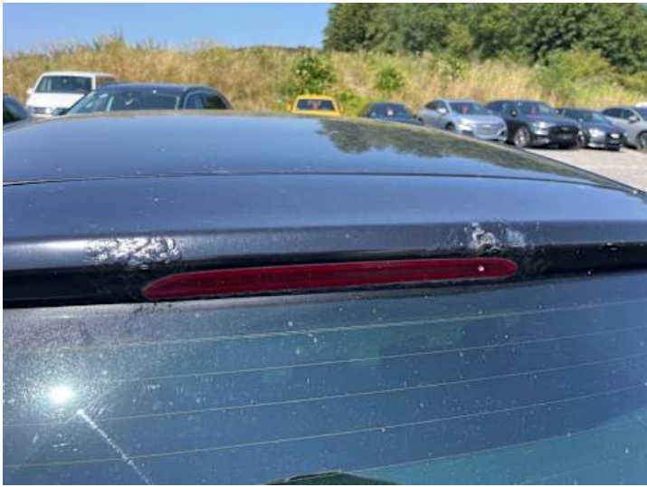
Heckklappe (Lackschaden, Rost)
