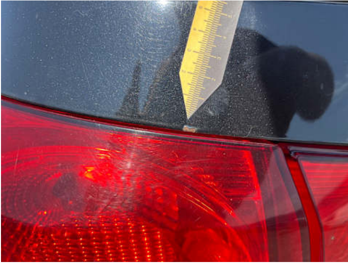
Heckklappe (Lackschaden, Rost)
