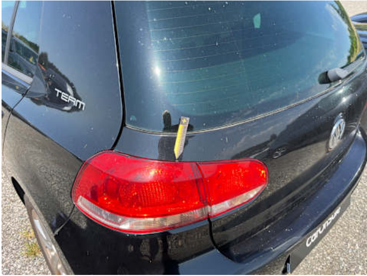
Heckklappe (Lackschaden, Rost)
