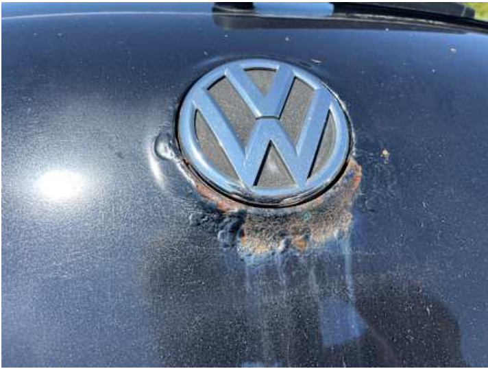
Heckklappe (Lackschaden, Rost)
