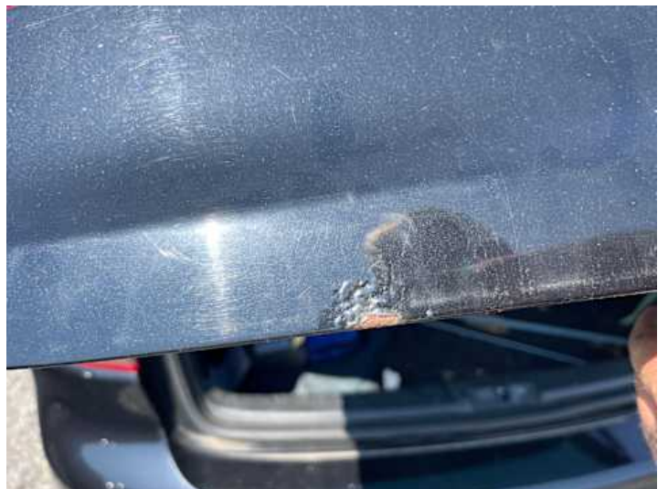
Heckklappe (Lackschaden, Rost)
