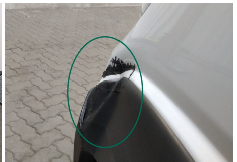
Kotflügel / Vorne Links / Delle
