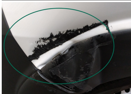
Kotflügel / Vorne Links / Delle
