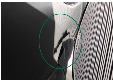
Kotflügel / Vorne Links / Delle
