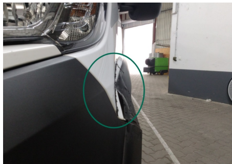
Kotflügel / Vorne Links / Delle
