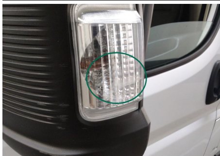
Blinker / Links / Kratzer
