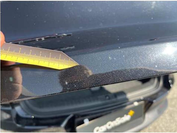
Heckklappe (Lackschaden, Rost)
