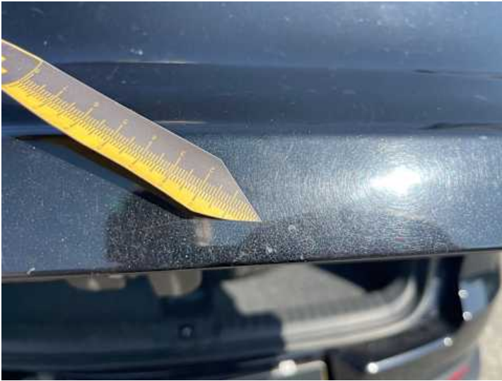
Heckklappe (Lackschaden, Rost)
