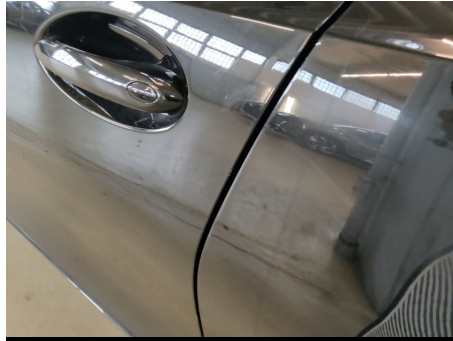
Tür / Vorne Links / Kratzer
