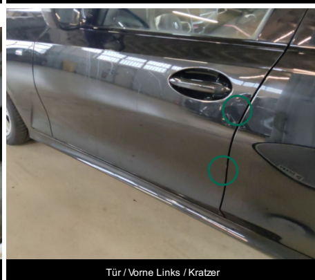
Tür / Vorne Links / Kratzer
