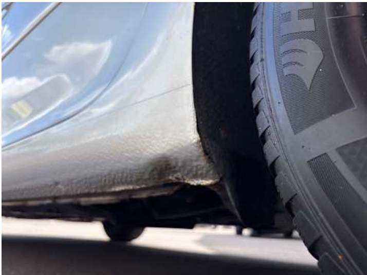
Schweller links (Lackschaden, Verformung, Rost)
