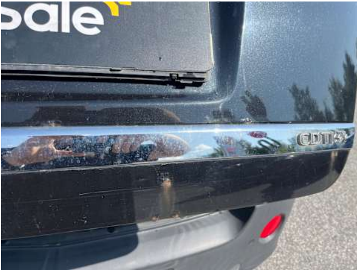
Heckklappe (Lackschaden, Rost)
