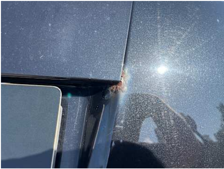
Heckklappe (Lackschaden, Rost)
