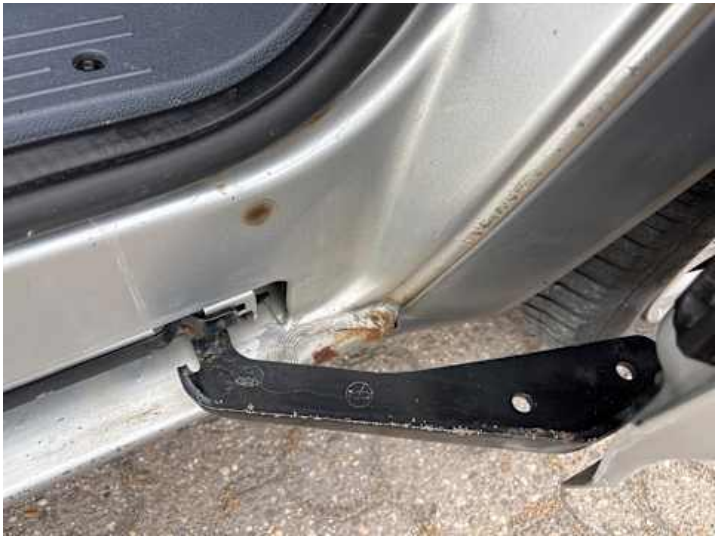
Schweller links (Lackschaden, Rost)
