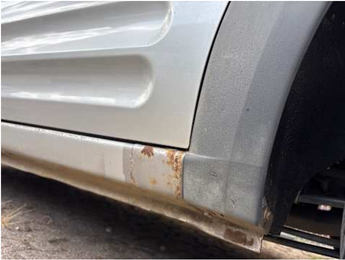
Schweller links (Lackschaden, Rost)
