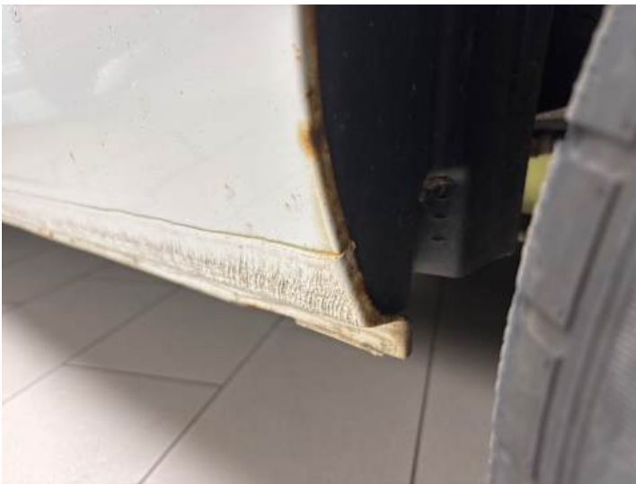
Schweller links (Lackschaden, Rost)
