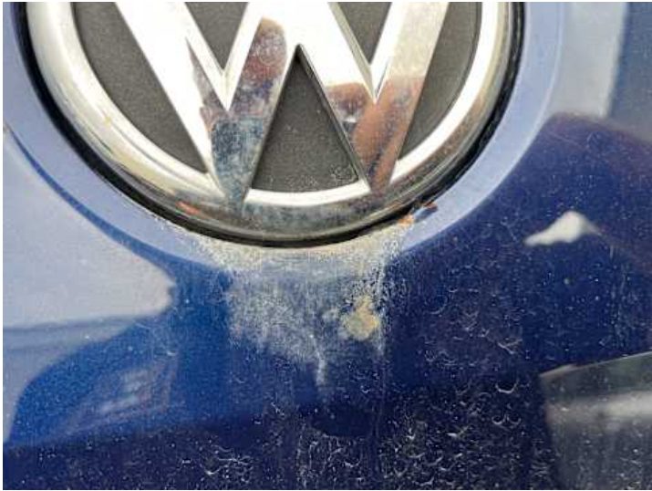
Heckklappe (Lackschaden, Rost)
