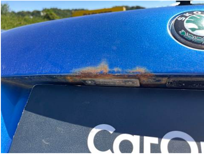
Heckklappe (Lackschaden, Rost)
