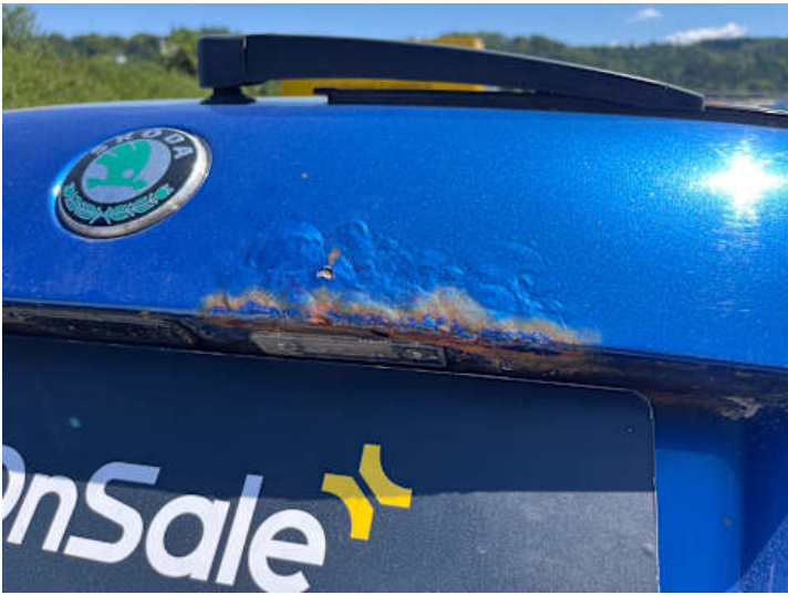
Heckklappe (Lackschaden, Rost)
