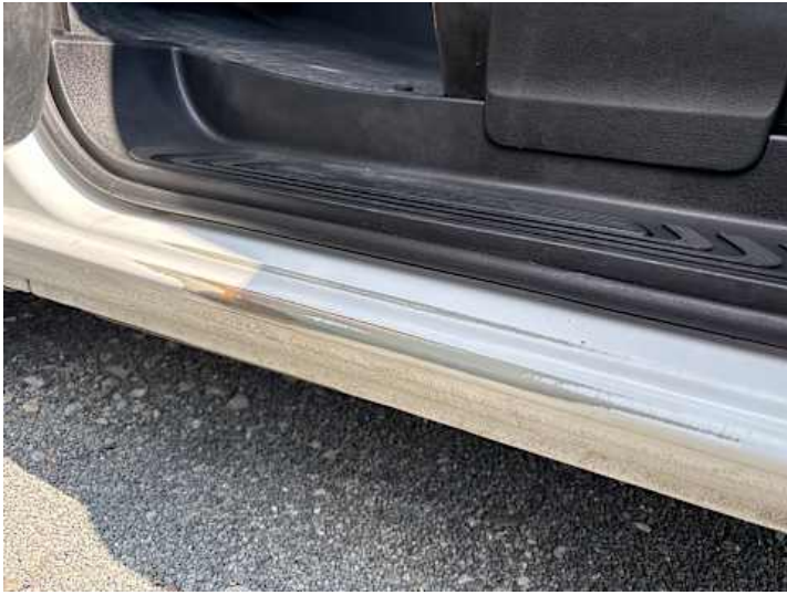
Schweller links (Lackschaden, Rost)
