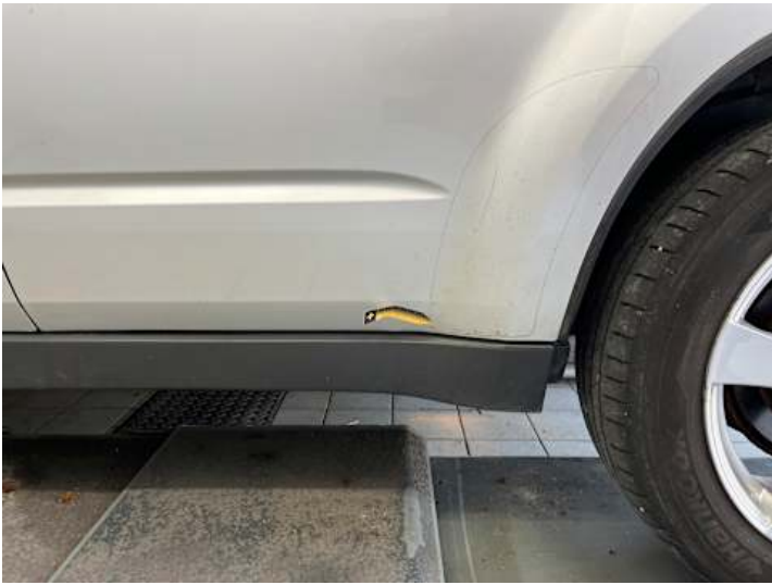
Türe hinten links (Lackschaden, Rost)
