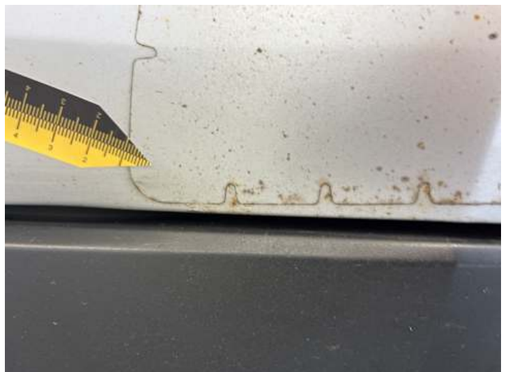
Türe hinten links (Lackschaden, Rost)
