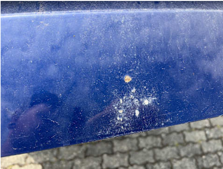
Heckklappe (Lackschaden, Rost)
