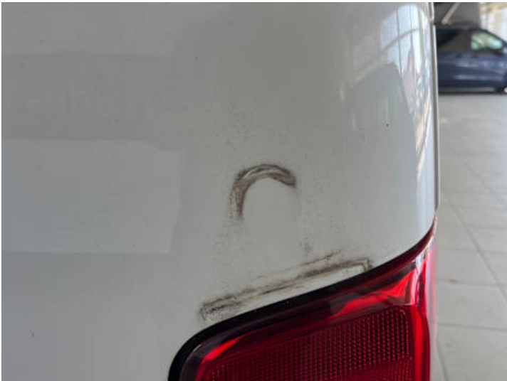
Heckklappe (Lackschaden, Rost)
