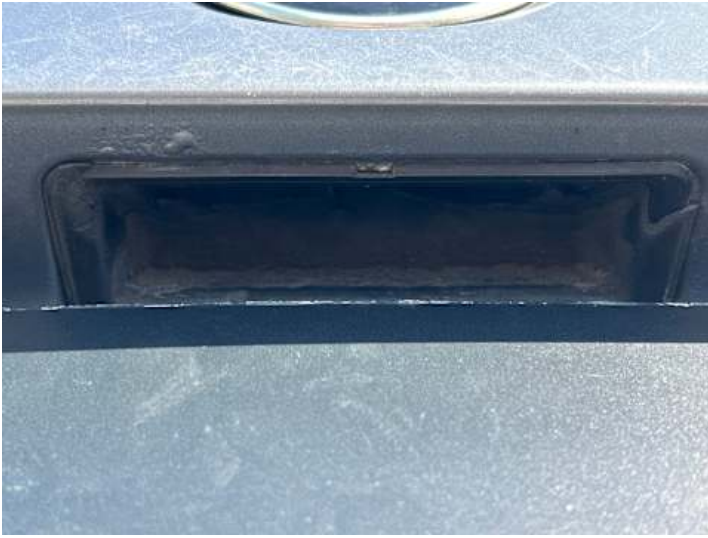
Heckklappe (Riss/Bruch, Rost)
