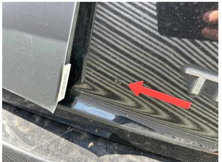
Heckklappe (Delle, Rost)
