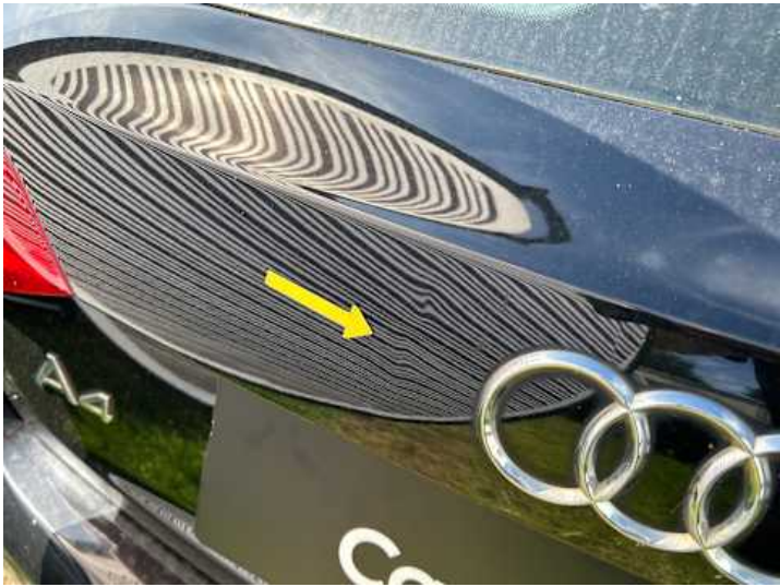
Heckklappe (Delle, Rost)
