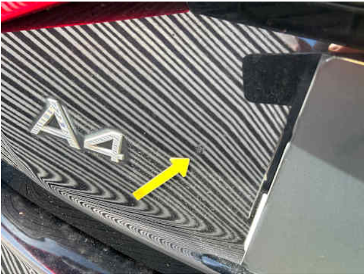
Heckklappe (Delle, Rost)
