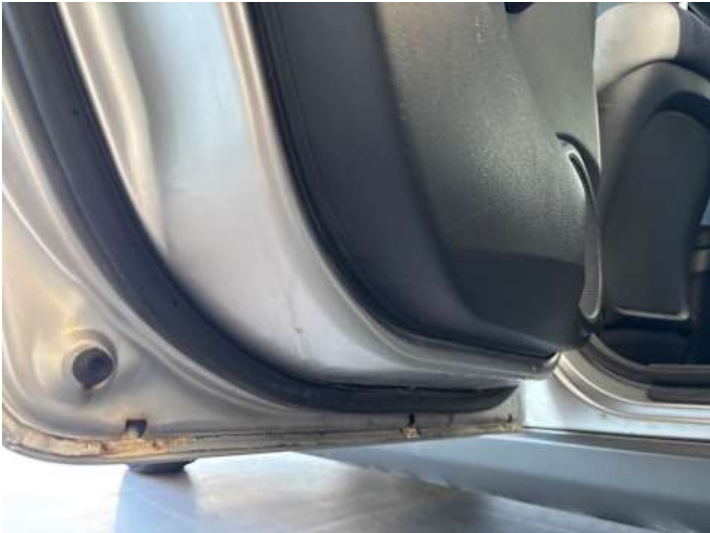
Türe hinten links (Lackschaden, Rost)
