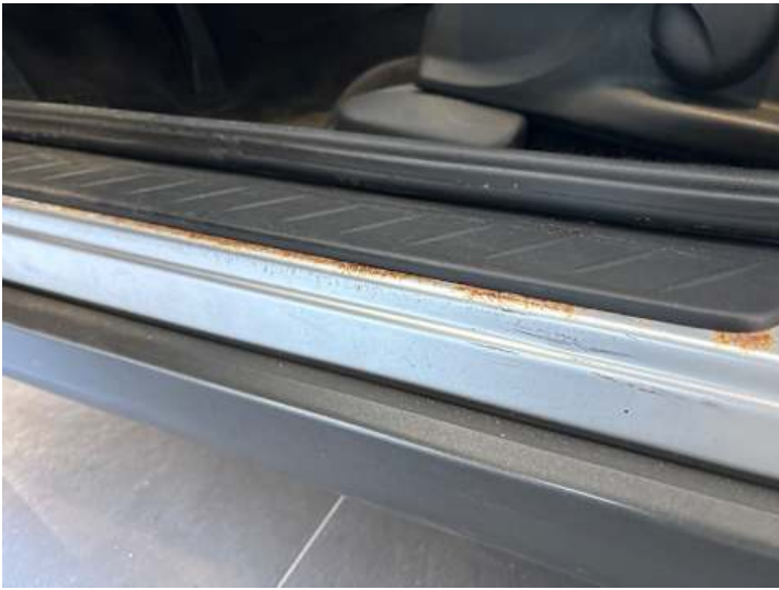
Schweller links (Lackschaden, Rost)
