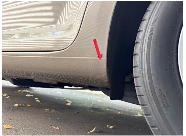
Schweller links (Lackschaden, Rost)
