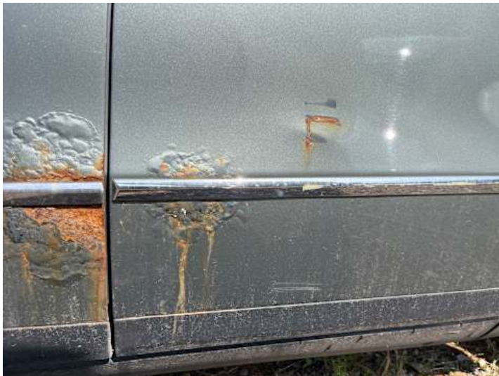
Türe hinten links (Lackschaden, Rost)
