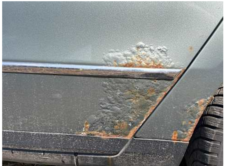
Türe hinten links (Lackschaden, Rost)
