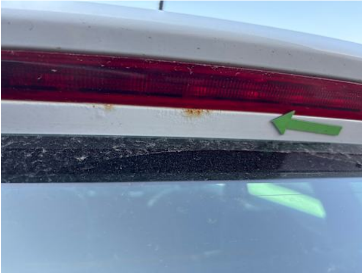
Heckklappe (Lackschaden, Rost)
