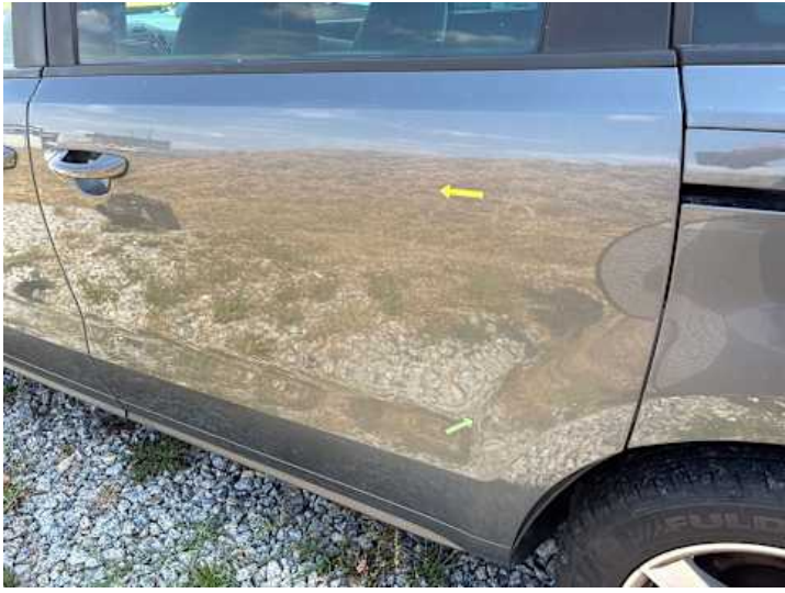
Türe hinten links (Delle, Rost)
