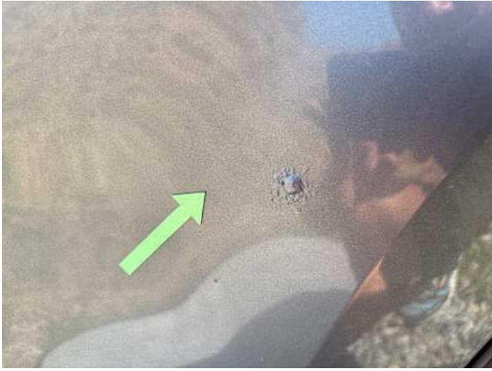
Türe hinten links (Delle, Rost)
