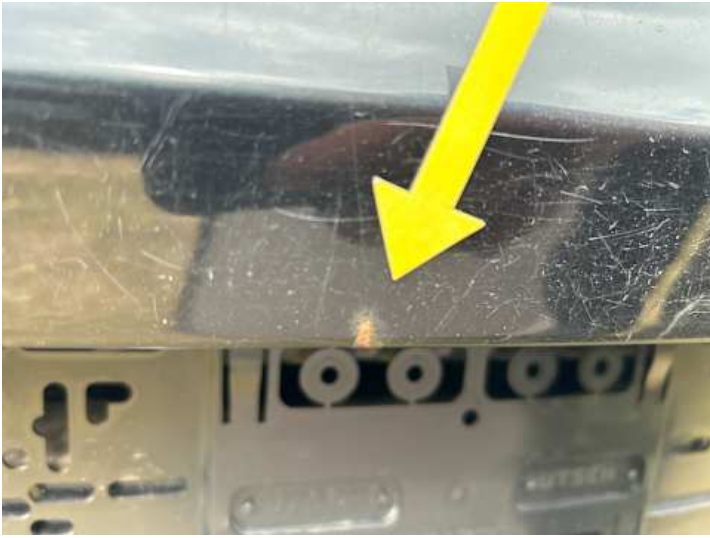
Heckklappe (Lackschaden, Rost)
