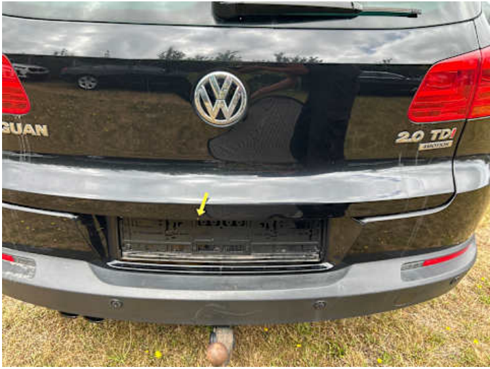
Heckklappe (Lackschaden, Rost)
