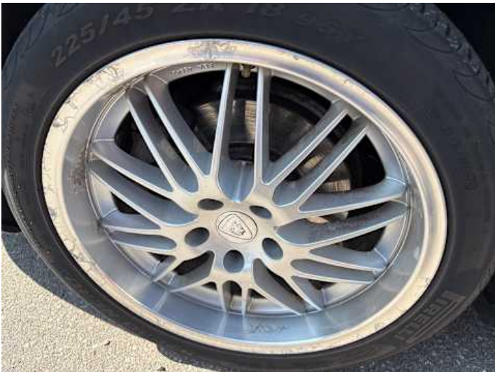
Wheel (Scratch , Rust )
