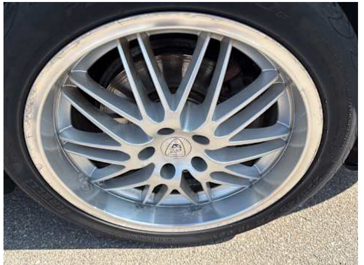
Wheel (Scratch , Rust )
