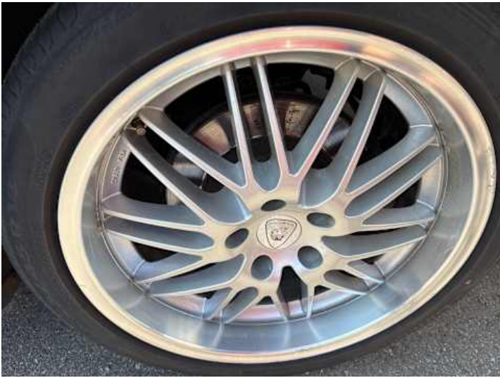
Wheel (Scratch , Rust )
