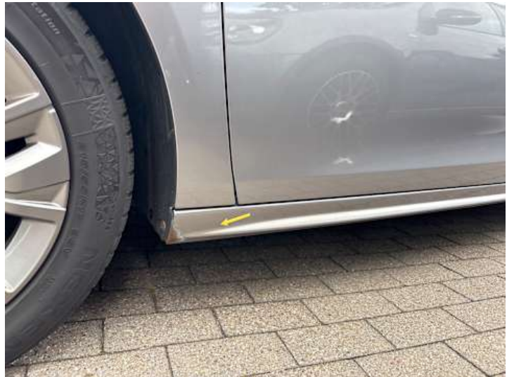
Schweller links (Lackschaden, Rost)
