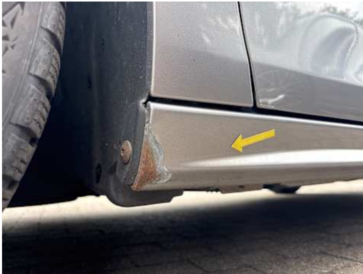
Schweller links (Lackschaden, Rost)
