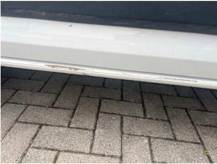
Schweller links (Lackschaden, Rost)
