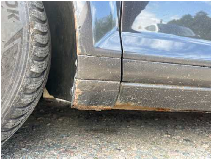
Schweller links (Lackschaden, Rost)
