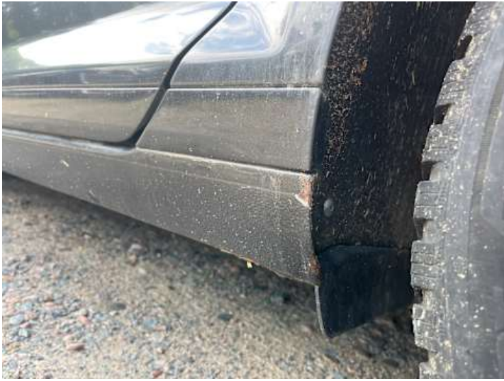
Schweller links (Lackschaden, Rost)
