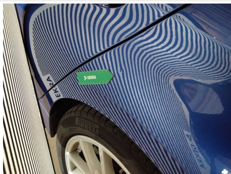
Kotflügel / Hinten Links / Delle
