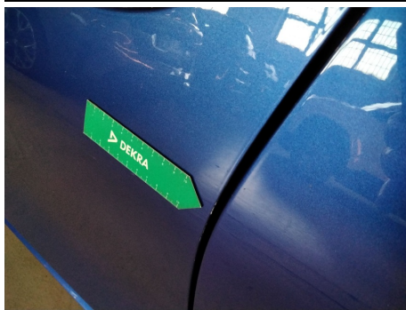
Tür / Vorne Links / Kratzer
