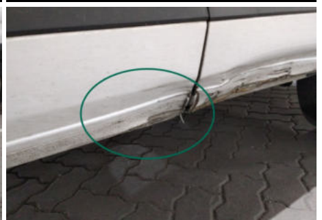
Schweller / Links / Delle
