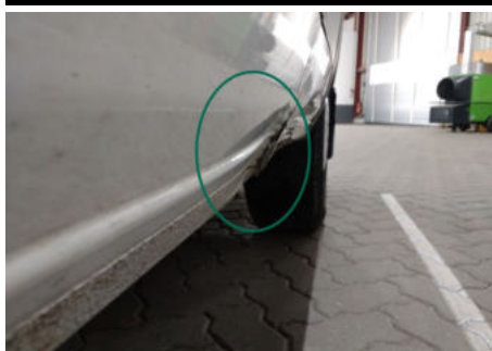
Schweller / Links / Delle
