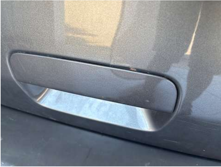
Heckklappe (Lackschaden, Rost)
