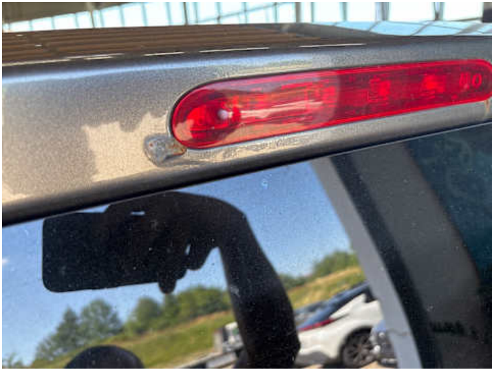
Heckklappe (Lackschaden, Rost)
