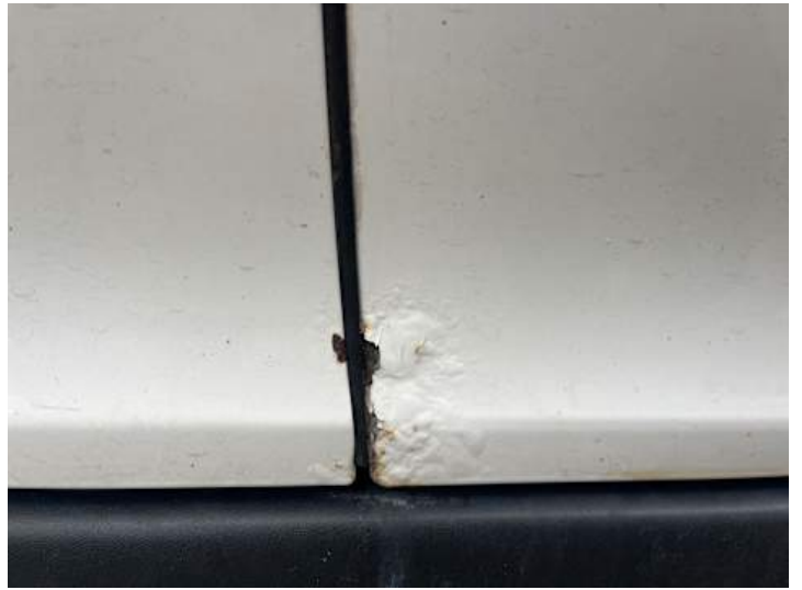
Türe hinten links (Lackschaden, Rost)
