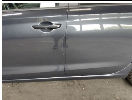
Tür / Vorne Links / Kratzer
