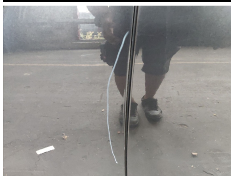
Tür / Vorne Links / Kratzer
