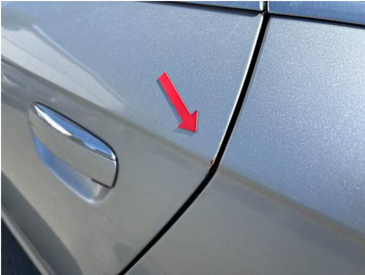
Türe hinten links (Lackschaden, Rost)
